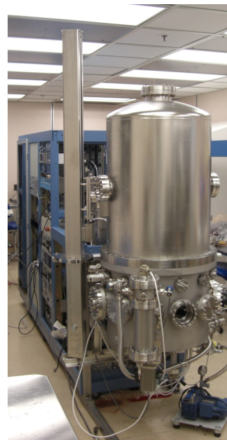
Figure 6: UHV multi-technique deposition facility.
