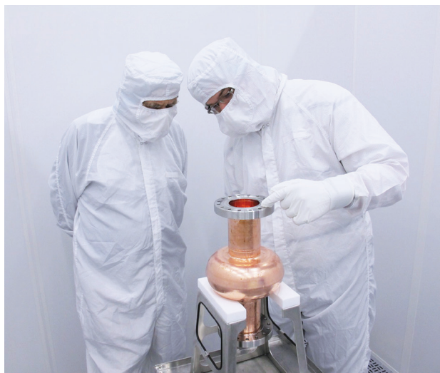
Larry Phillips (left) and Matthew Burton visually inspect a clean copper cavity which has been prepared for the HiPIMS process to apply a dense thin film of niobium on the inner surface of the cavity. Image: C. Reece, JLab
